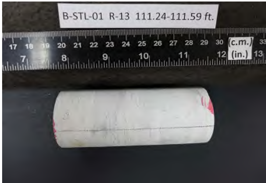
After cutting and grinding
