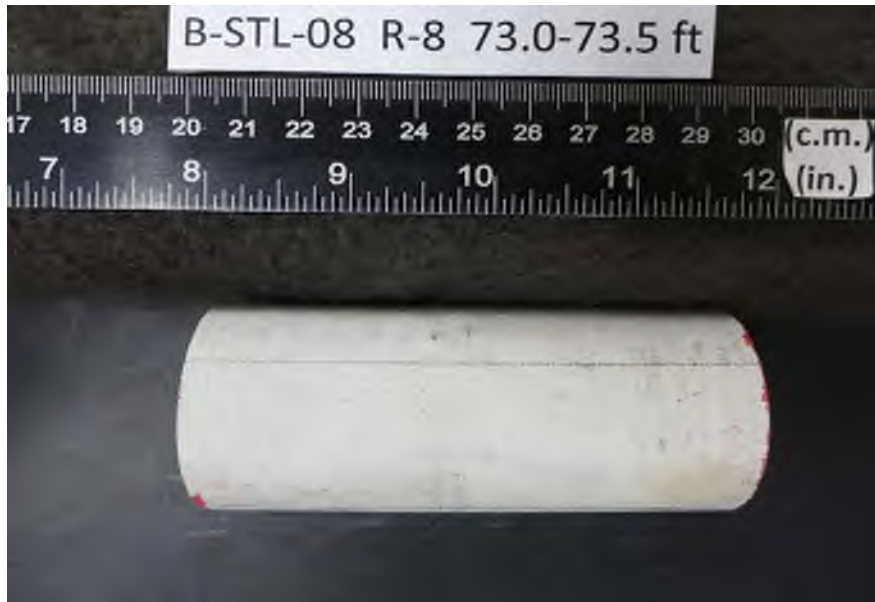
After cutting and grinding
