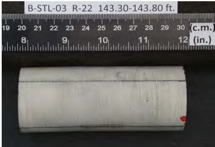
After cutting and grinding
