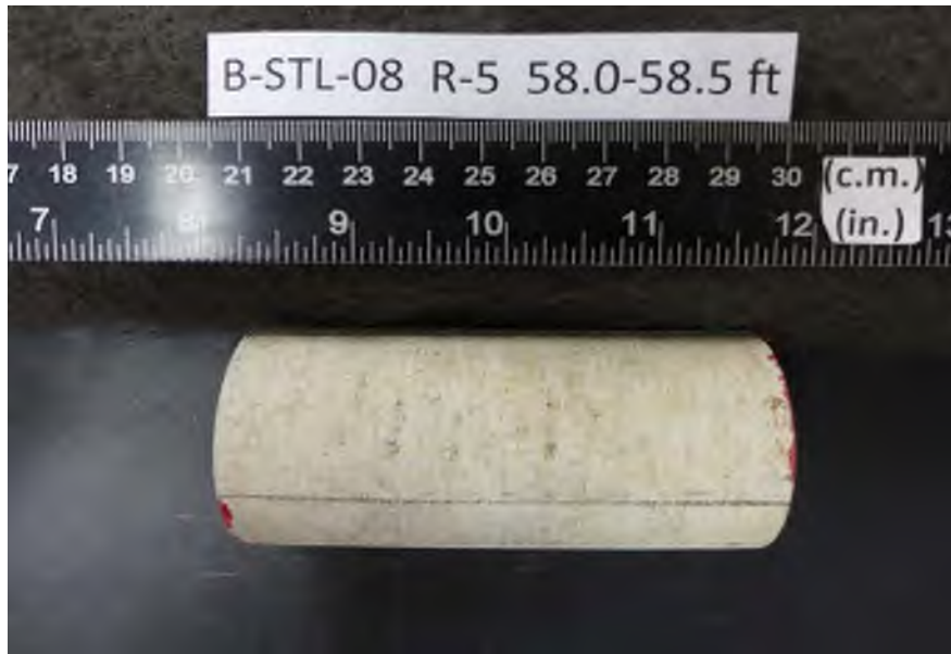
After cutting and grinding
