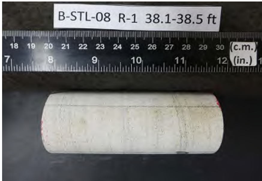
After cutting and grinding
